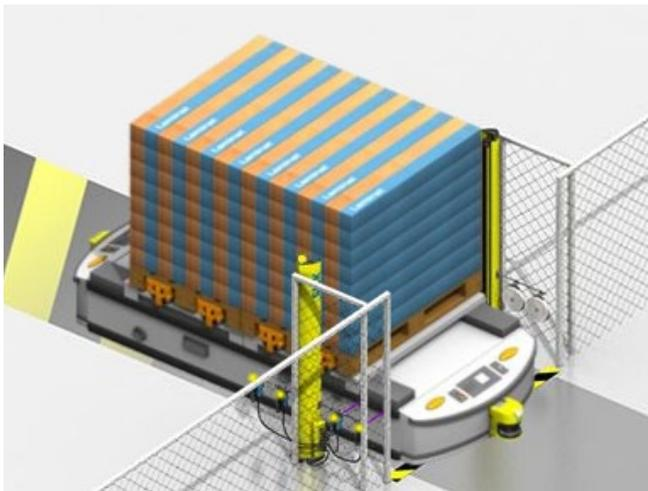
Entry/exit station with 4 muting sensors, the material can flow in both directions
