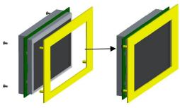
The product is installed from the back to front. 4\*M3 thread holes are reserved all around, and the hole position of the shell (refer to the left) is aligned with the thread hole, and the screw is screwed into the M3 specification. Note: the front touch panel of the product needs external reinforcement to prevent falling off in long time or complex environment!
